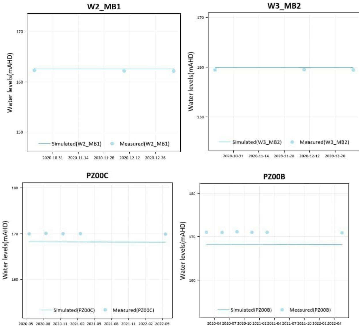
**Figure 2-10 Calibration Fit - Alluvium Bores**
