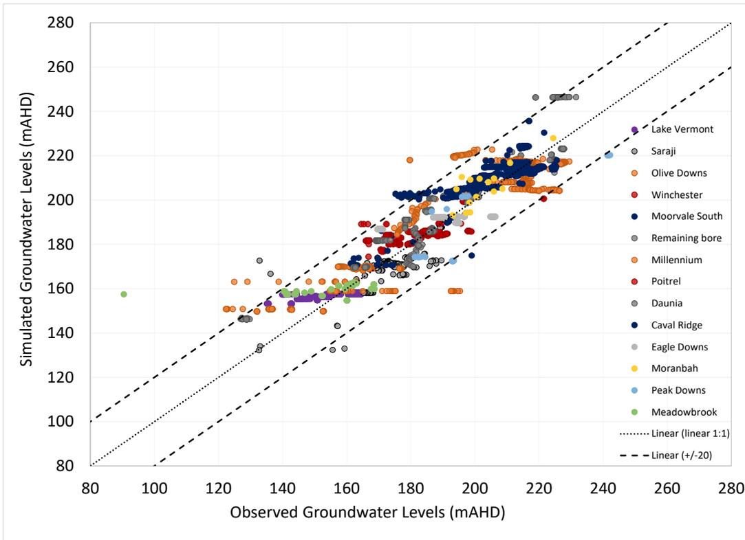
Figure 2-6 Calibration Scattergram – Modelled vs Observed Groundwater Levels (All Bores)
