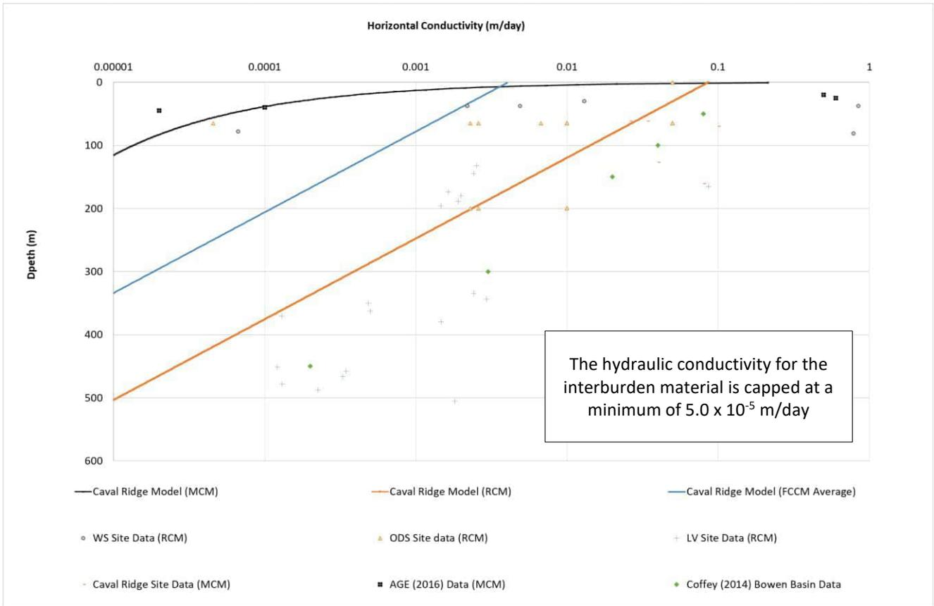
**Figure 2-13      Hydraulic Conductivity vs Depth – Interburden/Overburden**
