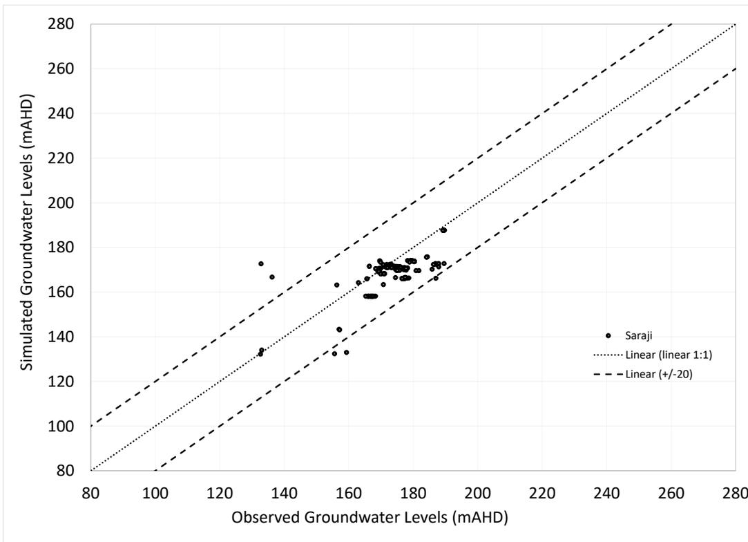
Figure 2-7 Calibration Scattergram – Modelled vs Observed Groundwater Levels (SEMLP Bores)
