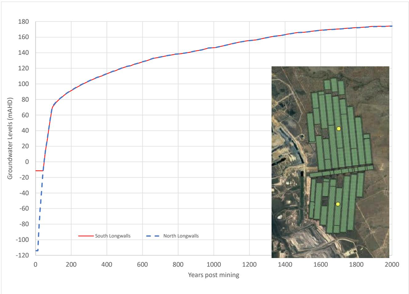
Figure 4-1 Predicted Groundwater Recovery within the SEMLP Workings
