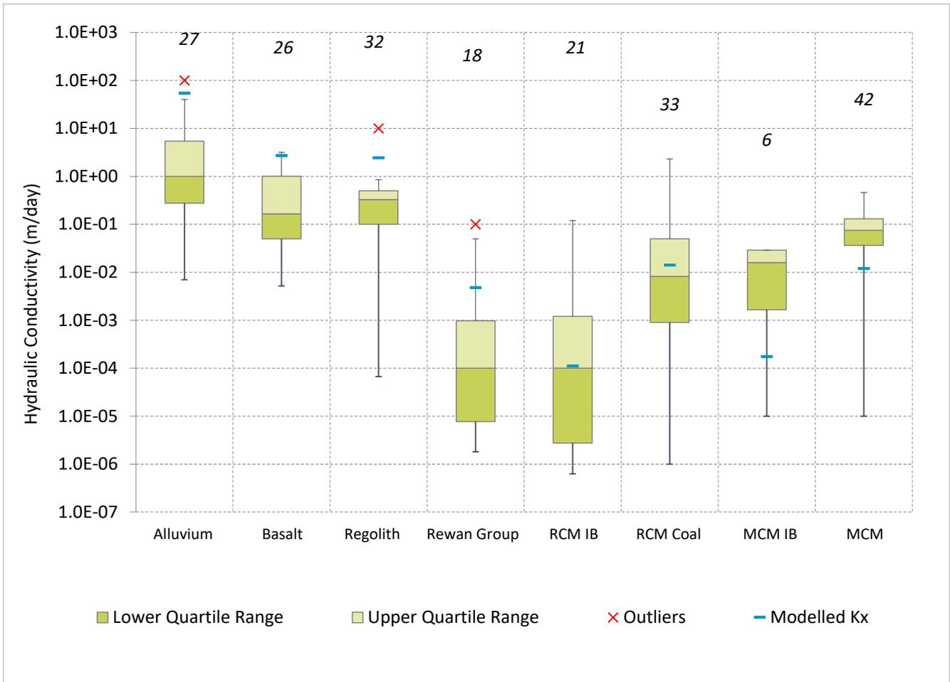
Figure 2-15 Hydraulic Parameters Estimates vs Best Calibrated Hydraulic Parameters
