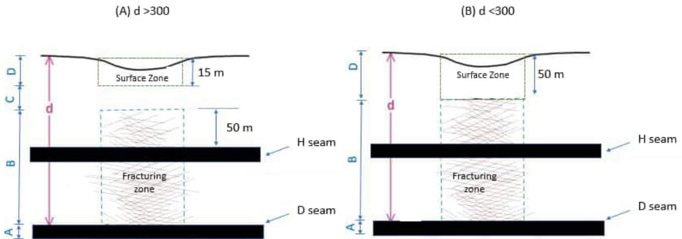
A = Mined zone, B = Fracture Zone, C = Constrained Zone, D = Surface cracking
