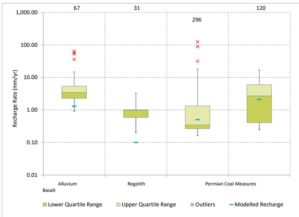
**Figure 2-16 CMB Recharge Estimates vs Modelled Recharge**
