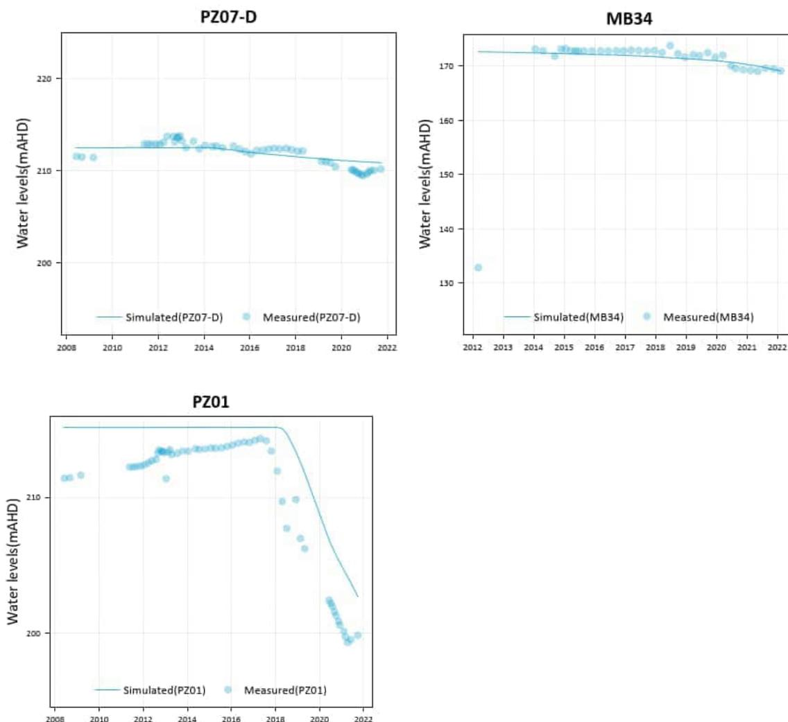
**Figure 2-11 Calibration Fit - Permian Bores (D,Q, P and H seams)**
