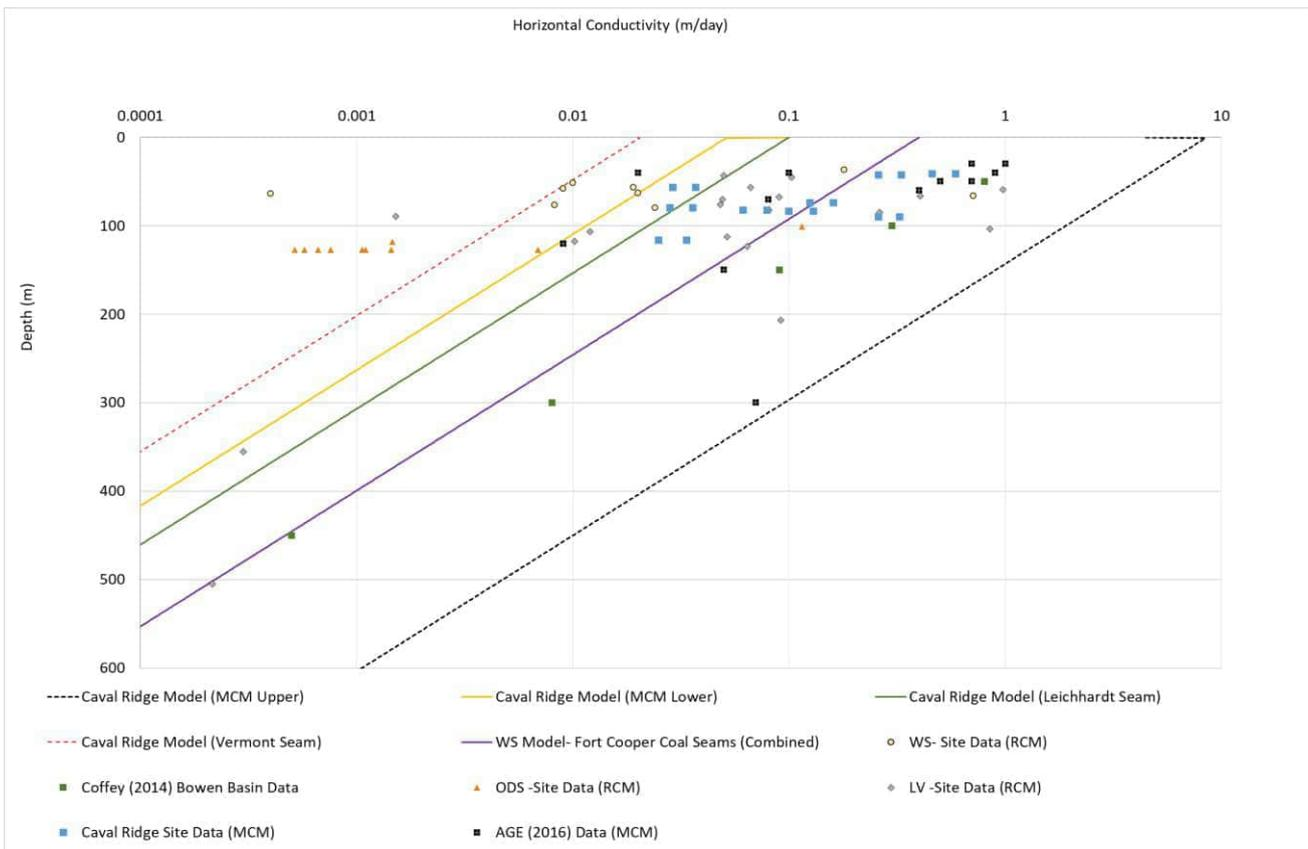
**Figure 2-14 Hydraulic Conductivity vs Depth – Coal**
